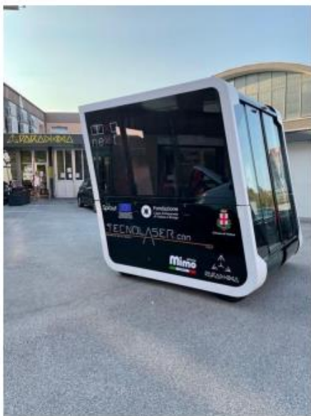
Figure 2: The NEXT system: modular pod for passengers and cargo hitching
